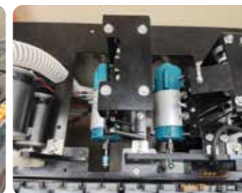
Japanese pure copper motor, Trimming & Cutting system
