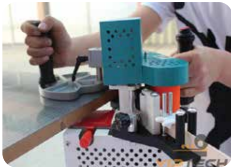
In the portable mode, any special-shaped plate can complete the edge banding work
