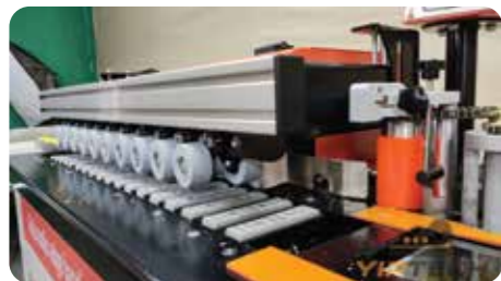
Automatic feeding system,Integrated die-cast aluminum alloy rubber wheels
