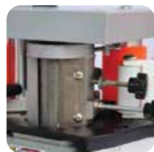
Double-sided gluing system
