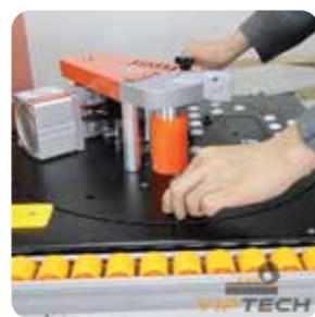
Double-sided gluing System
