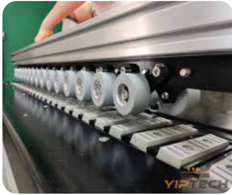
Integrated die-cast aluminum alloy rubber wheels, comparable to the configuration of large-scale edge banding machines, no degumming for ten years
