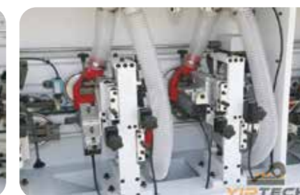
Sharp and Durable Diamond knives for Pre-milling
