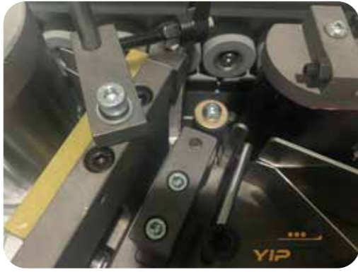
Cassette automatic tool setting to accurate fix the location edge banding
